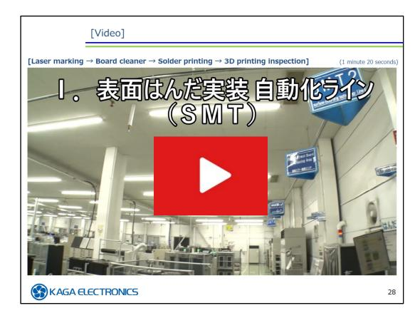
You will now be given a video tour. The first video is about the laser marking described previously. Laser marking is the process whereby each individual board is marked with a serial number.
