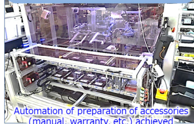
Automatic picking machine for instruction manual and other accessories
