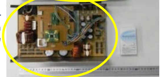
Sample power conditioner using an SiC substrate
